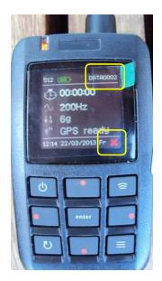
At the end of the acquisition, a red check will be shown in the lower right side of the display.
