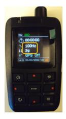
To set **sample rate frequency** go to "Main Menu" (button 9) and push down (button 8) till selecting "Parameters" (button 5):
