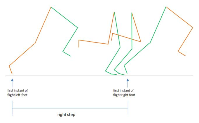
The first information returned by the software is the first flight phase subsequent to the take-off of the front foot.
